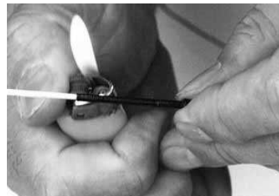
Burn the cut end with a light, paying attention to stay as far as possible from the string itself.
