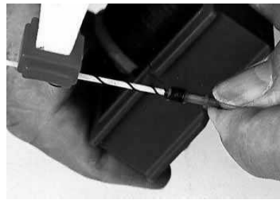
At the outer shoulder, the thread will return to the string through the free, out-going thread indentation.
